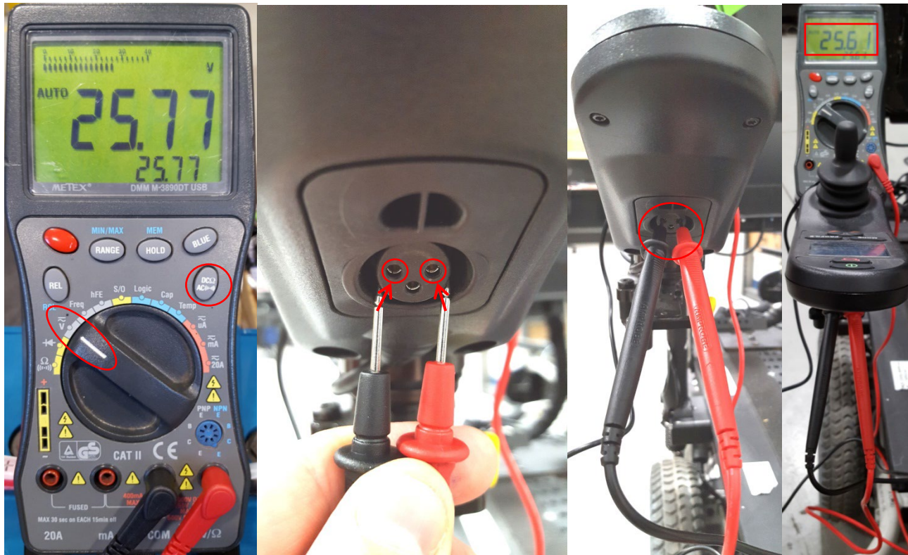
Probe connections from multimeter to joystick
