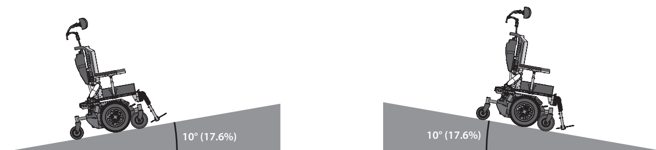
Figure 3. Do not use power wheelchair on slope steeper than 10°.
