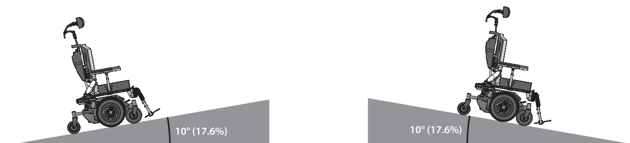
Figure 3. Do not use power wheelchair on slope steeper than 10°.
