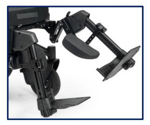
Leg Length1<br/>rangesSOFLHD12:  $12 \frac{1}{2}$ " -  $15 \frac{1}{2}$ " (320-395 mm)2SOFLHD12:  $12 \frac{1}{2}$ " -  $17 \frac{1}{2}$ " (320-445 mm)2SOFLHD14:  $14 \frac{1}{2}$ " -  $19 \frac{1}{2}$ " (370-495 mm)SOFLHD14:  $14 \frac{1}{2}$ " -  $19 \frac{1}{2}$ " (370-495 mm)Adjustment was made in 1" increments.Adjustment is made in \frac{1}{2}" increments.
