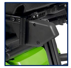
Both heavy duty footrests and manual/power elevating & articulating legrest adjust the same way and offer settings of 60° and 70°.
